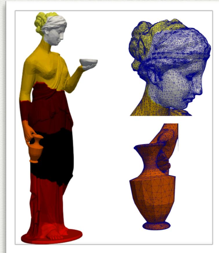
Partitioning of finite element mesh.
