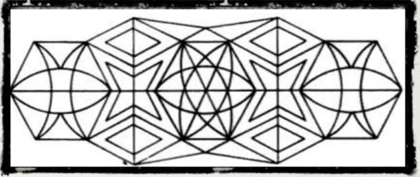
J.B. Listing's single stroke drawing. There are only two nodes of odd degree, lying at the end of the horizontal line [6].
