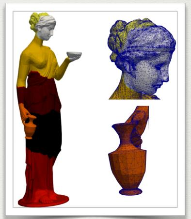
Partitioning of finite element mesh.
