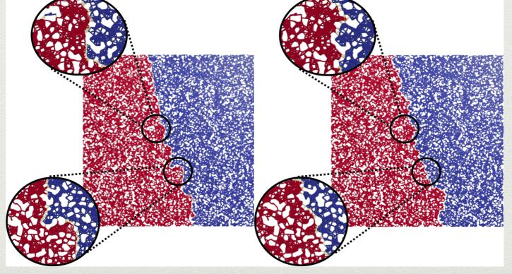
Refining a random geometric graph rom the 10th DIMACS Implementation Challenge. Selected close-ups are illustrated. In the top ones the removal of isolated partition islands, present in the standard spectral bisection, is depicted. In the bottom ones, the removal of redundant cut edges is presented [2].
